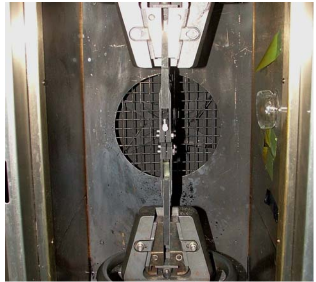
Fig. 11 Pull-out equipment: the tensile tools are clamped and installed in the environmental chamber
